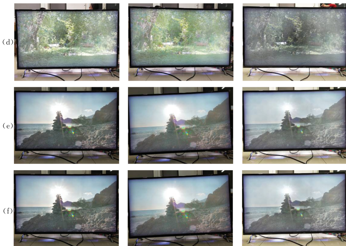
图 8 6 副 HDR 显示器显示的测试图像.本文提出的算法(左),Seetzen 等 [3] 的算法(中),Narwaria 等 [14] 的算法(右)。 Fig.8 Six test images displayed on the HDR display. The algorithm by this paper (left), the algorithm by Seetzen et al [3] (middle), the algorithm by Narwaria et al [14] (right).
